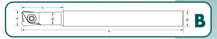
IEM B cutter bodies are used with CIB (back draft) and CIF (flat bottom) inserts. However, CIF and CIB inserts in sizes .0250, .0312, .0375, 6, 8, and 10 fit IEM R (round) cutter bodies.
